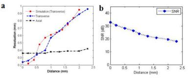
Fig. 2. Performance of this system. (a) Axial and transverse resolutions versus target depth. (b) Signal-to-noise ratio (SNR) versus target depth.
