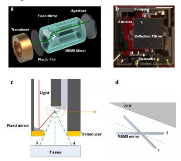
Fig. 1. Schematic representation of the MEMS probe. (a) 3D rendering of the probe (b) Photograph of the MEMS mirror with four actuators and five pads bonded with gold wire (Media 1). (c) Schematic of the miniaturized probe. A wedge-shaped mirror plated with aluminum is fixed in position to redirect the light beam to the MEMS mirror. (d) The MEMS mirror is fixed on a ramp with an angle of  $22.5^{\circ}$
